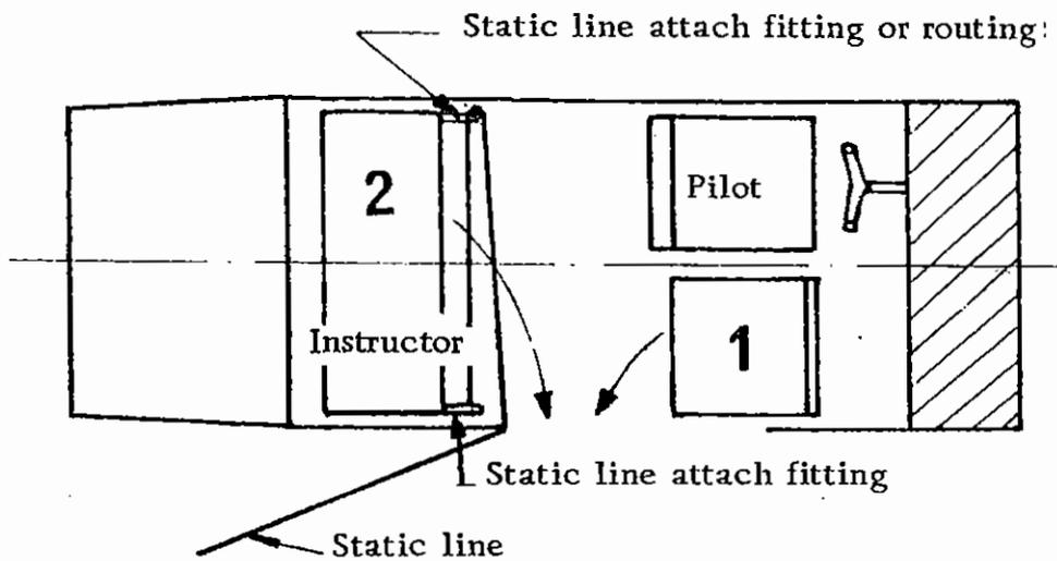
Depending on their length, static lines are attached to either fitting on front feet of skydiver rear bench-type seat.
