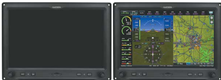
G3X Touch Full-Screen Reversionary Mode (Failed PFD)
