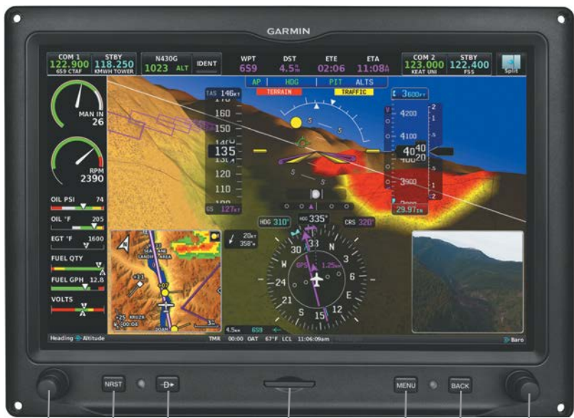
Left Knob Nearest Button Direct-to Button SD Card Slot Menu Button Back Button Right Knob
