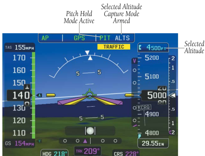
Pitch Hold & Selected Altitude Capture Modes
