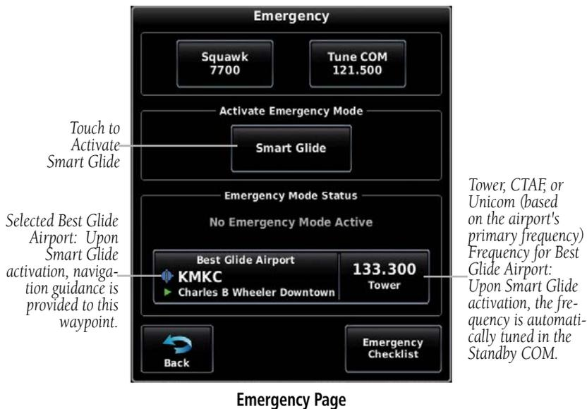
When Smart Glide is active and the Emergency Data Bar button is not displayed, the Status Bar displays a **Glide** button. Touch **Glide** to display the Emergency Page.
