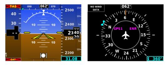
1. Use an alternate source of outside air temperature to calculate true airspeed, density altitude, and winds.
